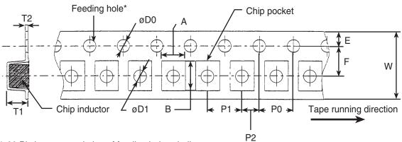
$^{*}$  20 Pitches accumulation of feeding holes shall be 80  $\pm$  0.15 mm.
